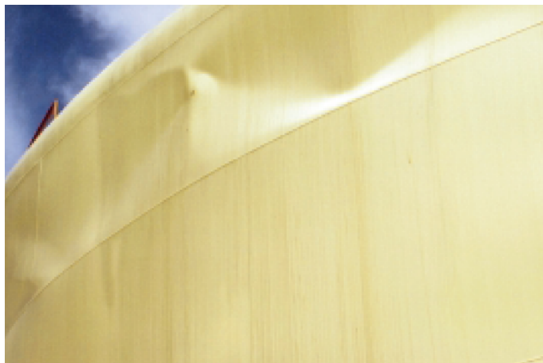
Figure B.5-7 – Sloshing damage to upper shell of a tank. San Fernando (California) earthquake 1971, magnitude 6.6.
