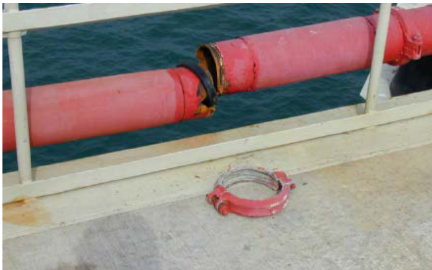
Figure B.6-4 – Support break. Peru 2001 M 8.4.
